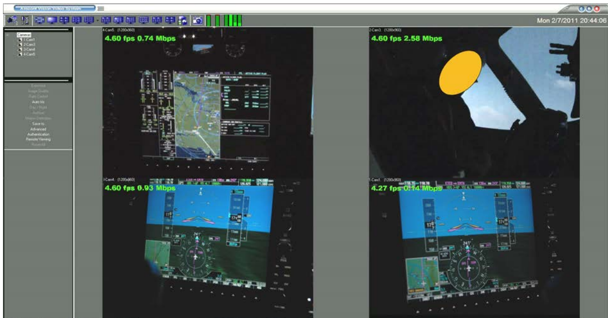
Figure 15. Four camera views of Cessna Mustang simulator cockpit. Starting from top left rotating clockwise: MFD; view of pilot; pilot's PFD; co-pilot's PFD.
