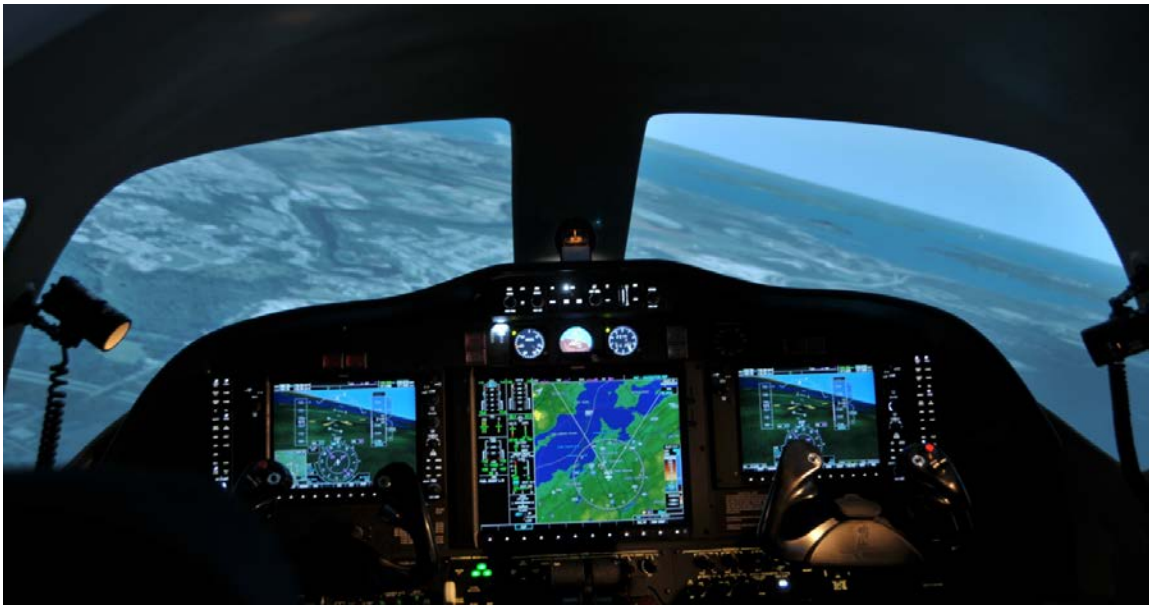
Figure 6. Simulator G1000 avionics suite and out-the-window view.
