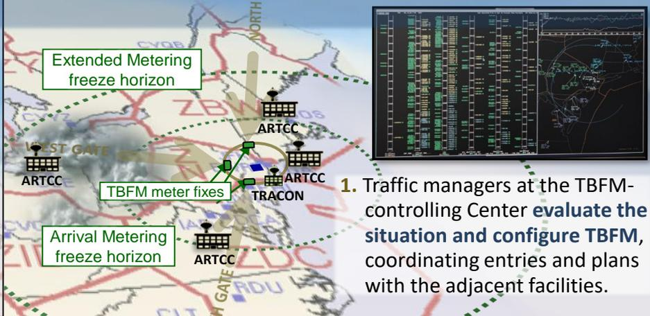
1. Traffic managers at the TBFM-controlling Center **evaluate the situation and configure TBFM**, coordinating entries and plans with the adjacent facilities.
