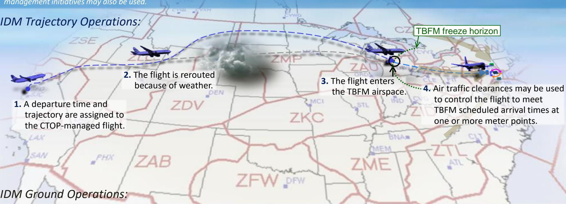
1. A departure time and trajectory are assigned to the CTOP-managed flight.
