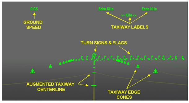
Figure 2. T-NASA Head-Up Display (HUD)
