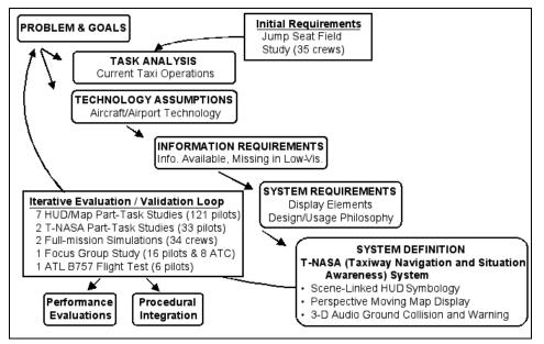
Figure 4. T-NASA Human-Centered Design Process
