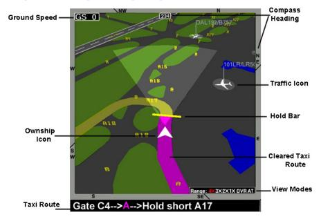
Figure 3. T-NASA Electronic Moving Map (EMM; showing track-up perspective view)
