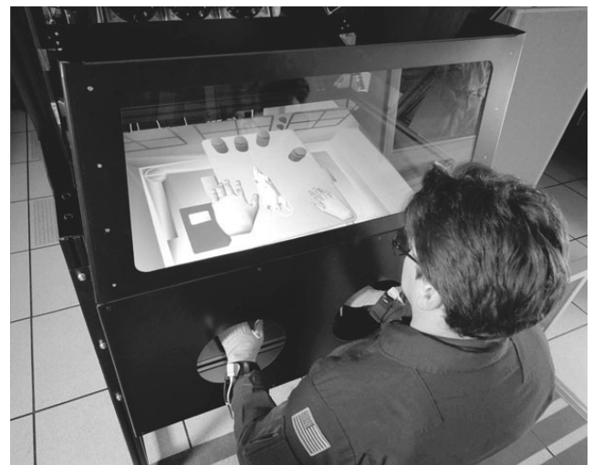
Figure 2: A Stereoscopic Display Station uses two digital projectors and polarized optics to provide an ultra-high resolution immersive environment for the VGX of about the same size as the working space of the Life Sciences Glovebox Facility. An operator reaches under the projected screen to see a virtual representation of his/her hands and the inside of the glovebox.
