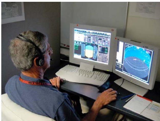
Figure 6: Flight deck interface to engage airborne spacing. An example desktop pilot station is shown on the bottom of the page. The CDTI is located on the right display. The data link interface and spacing panel are located together with the primary flight displays, the FMS and the Mode control panel on the left display.
