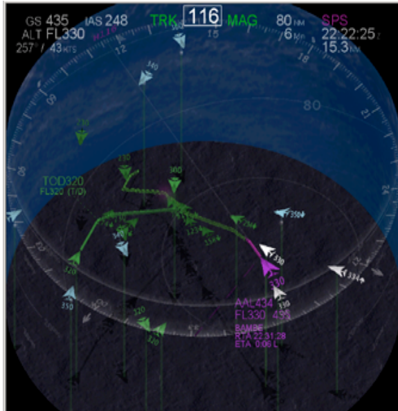
Figure 1. 3D CSD. To view pictures in color or to download a demo ( http://human-factors.arc.nasa.gov/ihh/cdti/download.html ).
