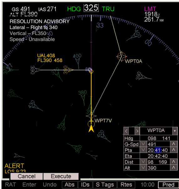
Figure 3. Conflict resolution agent suggesting a lateral maneuver. The flight crew may select and execute the maneuver by pressing the ‘Execute’ button.
