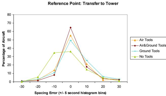
Figure 6. Spacing accuracy for aircraft in coordinated flows.
