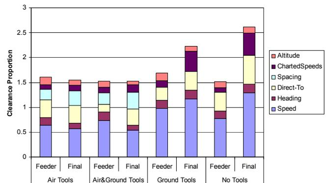
Figure 5. Relative proportions of maneuver clearances by controller, condition, and type.
