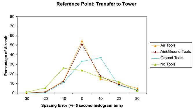
Figure 7. Spacing accuracy for aircraft in uncoordinated flows.
