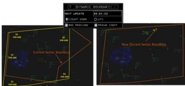
Figure 3. Radar Controller Boundary Change Preview Tool
