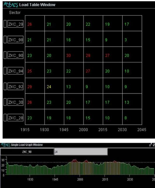
Figure 2. Prototype Traffic Load/Complexity Table/Graphs
