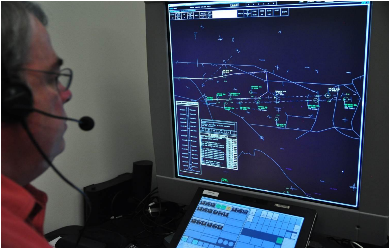
Figure 3 Experimental air traffic control station at NASA Ames with CMS controller tools
