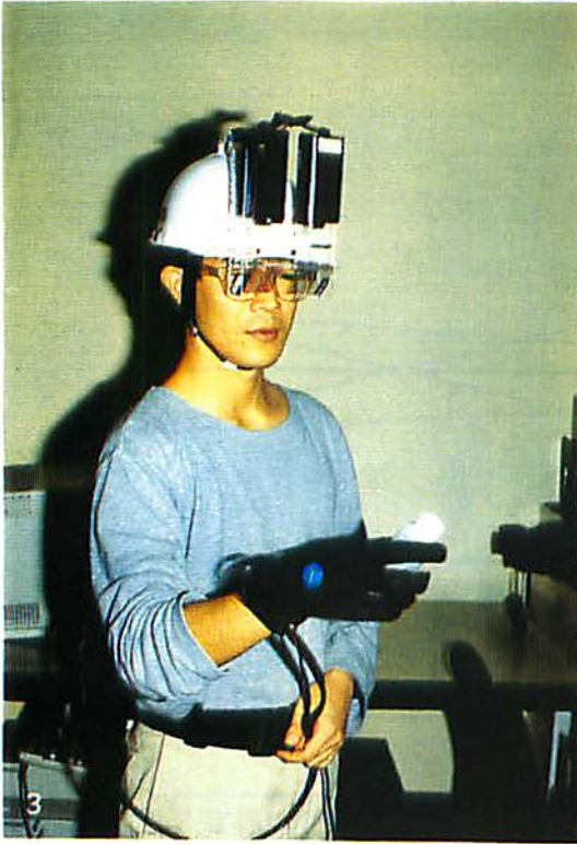
Fig. 3. See-through, head-mounted, virtual image, stereoscopic display that allows the user to interact with virtual objects synthesized by computer graphics which are superimposed in his field of vision. 39 The user's hand position is tracked electromagnetically and its shape is measured by the VPL DataGlove 30 . (Photograph courtesy of Michitaka Hirose.)
