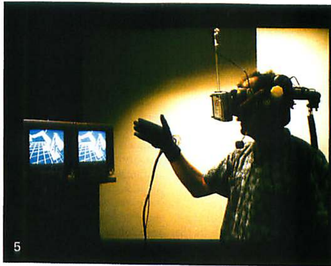
Fig. 5. This head-mounted, stereo, virtual environment display system at the Ames Research Center Advanced Display and Spatial Perception Laboratory is being used to control a remote PUMA robot in the Ames Robotics Laboratory. The simulation update rate varies from 12 to 30 Hz, depending on the complexity of the graphics. A local kinematic simulation of the remote work site aids the operator in planning complex movements and visualizing kinematic and operational constraints on the motion of the end effector. (Photography courtesy of NASA.)
