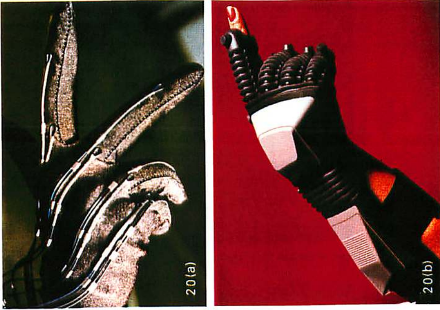
Fig. 20. Less bulky hand shape measuring instruments using flexible sensors (top panel; courtesy of VPL, Redwood City, California; bottom panel; courtesy of W. Industries, Leicester, U.K.).
