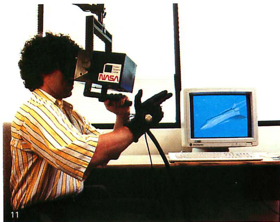
Fig. 11. Virtual environment technology may assist visualization of the results of aerodynamic simulations. Here a DataGlove is used to control the position of a "virtual" source of smoke in a wind-tunnel simulation so the operator can visualize the local pattern of air flow. In this application the operator uses a viewing device incorporating TV monitors 104 to present a stereo view of the smoke trail around the test model also shown in the desk-top display on the table. 105 (Photograph courtesy of NASA.)
