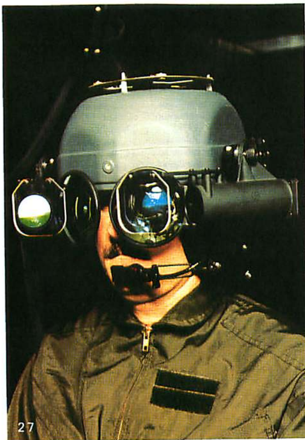
Fig. 27. Though very expensive, the CAE Fiber Optic Helmet Mounted display, FOHUD, is probably the best head-mounted, virtual environment system. It can present an overall visual field 162^\circ \times 83.5^\circ with 5 arcmin resolution with a high resolution inset of 24^\circ \times 18^\circ of 1.5 arcmin resolution. It has a bright display, 30 foot-Lambert, and a fast, optical head-tracker, 60 Hz sampling, with accelerometer augmentation. (Photograph courtesy of CAE Electronics, Montreal, Canada.)
