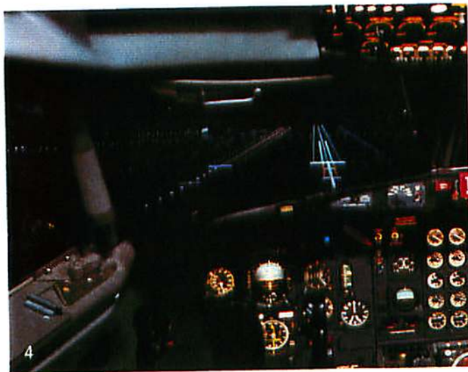
Fig. 4. View through the cockpit of a 727 simulator at the Ames Research Center which is used for human factors research. A simulated night flying environment is visible out the forward cockpit window. (Photograph courtesy of NASA.)
