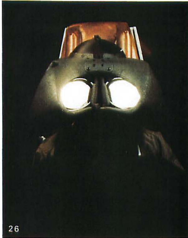
Fig. 26. Visually Coupled Airborne Systems Simulator of the Armstrong Aerospace Medical Research Laboratory of Wright-Patterson Air Force Base can present a wide field-of-view stereo display ( 120^\circ \times 60^\circ ) which is updated at up to 20 Hz. Head position is measured electromagnetically and may be recorded at a slower rate. Visual pixel resolution 3.75 arcmin/pixel. (Photograph courtesy of AAMRL, WPAFB.)
