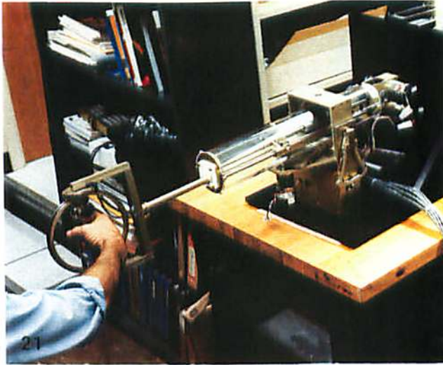
Fig. 21. A six degree of freedom force reflecting joystick. 123 (Photograph courtesy of JPL, Pasadena, California.)
