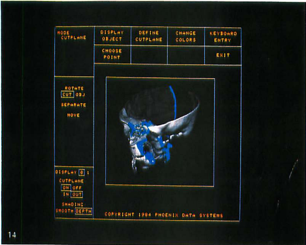
Fig. 14. Successive CAT scan X-ray images may be digitized and used to synthesize a volumetric data set which then may be electronically processed to identify specific tissue. Here bone is isolated from the rest of the data set and presents a striking image that even non-radiologists may be tempted to interpret. Forthcoming hardware will give physicians access to this type of volumetric imagery for the cost of an expensive car. (Photograph courtesy of Octree Corporation, Cupertino, California.)
