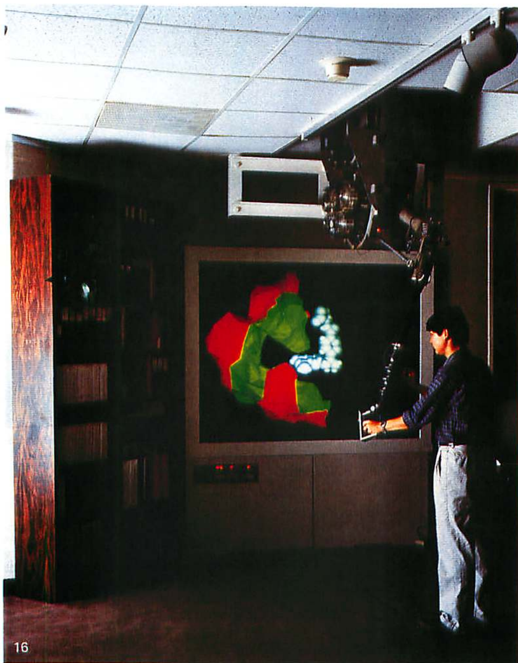
Fig. 16. Researcher at the University of North Carolina uses a multidegree-of-freedom manipulator to maneuver a computer graphics model of a drug molecule to find binding sites on a larger molecule. A dynamic simulation of the binding forces is computed in real time so the user can feel these forces through the force-reflecting manipulator and use this feel to identify the position and orientation of a binding site. (Photograph courtesy of University of North Carolina, Department of Computer Science.)
