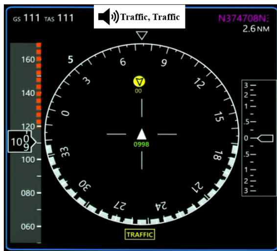
Fig. 7 Example of a TA. The advisory displays a caution-level icon and text banner. The “Traffic, Traffic” cue is provided audibly.
