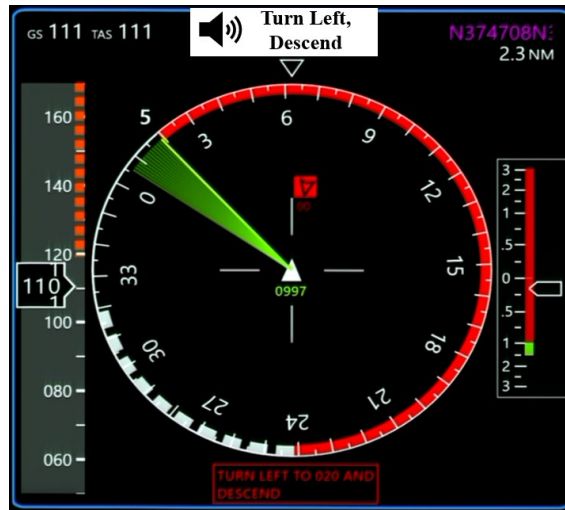
Fig. 6 Example of a Blended RA, which includes the RA icon, text banner, and red (avoidance) and green (target) horizontal and vertical banding. The “Turn Left and Descend” cue is provided audibly.
