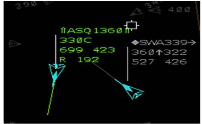
Figure 11. Scripted conflict that resulted in a TSAFE vector for ASQ1360 and vector for SWA339 in transition.
