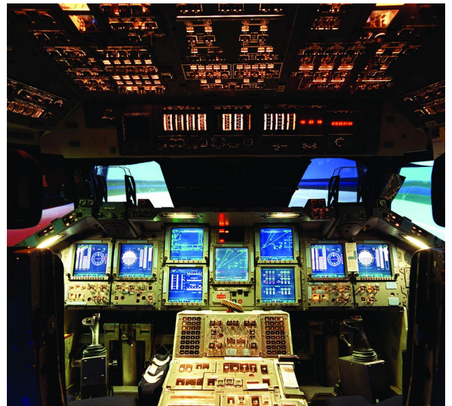
Figure 3: Updated space shuttle cockpit with LCD screens. Nine of the LCDs are in the forward part of the cockpit, as shown here. The remaining two are in the aft section of the cockpit.
