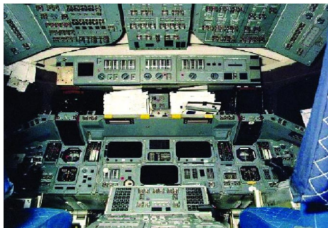
Figure 1: Original space shuttle cockpit. Three of the CRTs are in the forward section of the cockpit, as shown here. The fourth CRT is in the aft section of the cockpit.
