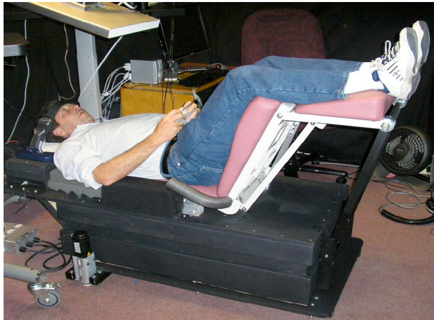
Figure 4. Ames Research Center's Fixed-Base Vibration Platform. Display and response device are from the previous Adelstein et al. (2009) study.
