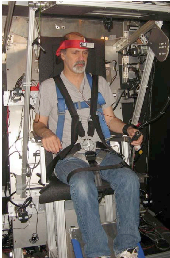
Figure 6. Vibration platform and chair in the Ames Research Center 20-G Centrifuge cab.
