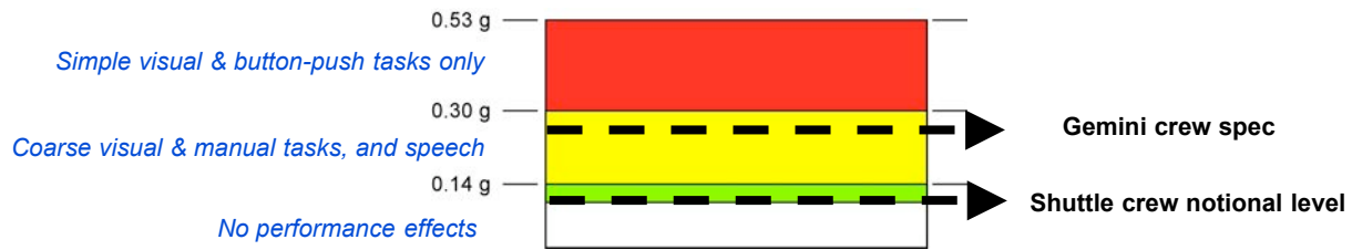
Figure 3. Human performance limits from Vykukal and Dolkas (1966) with Gemini specification (0.25 g) and Shuttle notional level (0.1 g measured on the flight deck, inside the console) for comparison.
