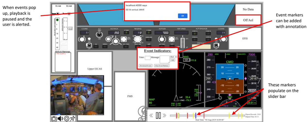
Figure 3: Pictured above is an 'Event Indicator' which are key events in flight that pause the playback and alert the user. Other event indicators are colored bars in the controller component below. By hovering over them the user can read their annotation.
