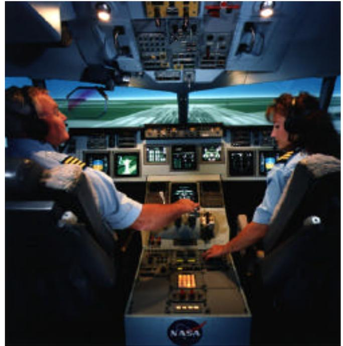
**Figure 4: Advanced Concepts Flight Simulator (ACFS) at NASA Ames Research Center**
