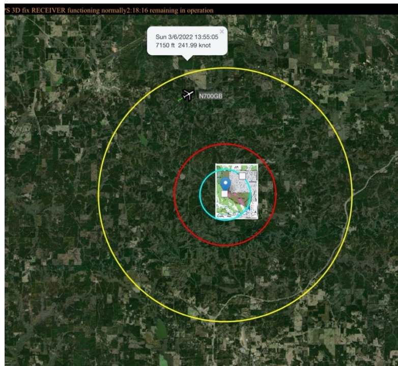
Fig. 6 An example of the display on the first prototype of the UASP-kit, with a cylindrical operational volume (cyan) the center of which is marked with a placemark on a fire-operations map, alerting rings (yellow and red), and an aircraft flying above the 5nm yellow boundary.
