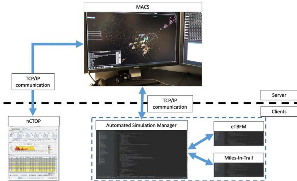
**Figure 12: System architecture of automated simulation capability (TMIAutoSim)**
