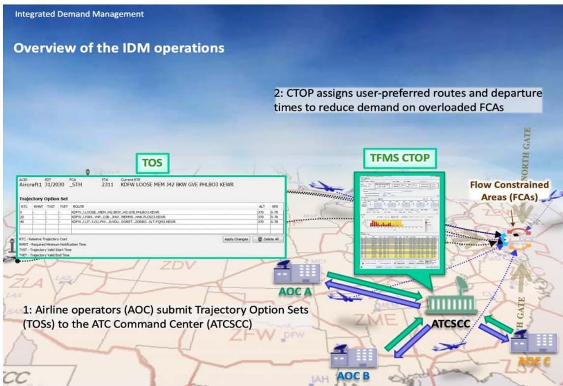
Figure 1: Schematic overview of tested IDM CTOP operations
