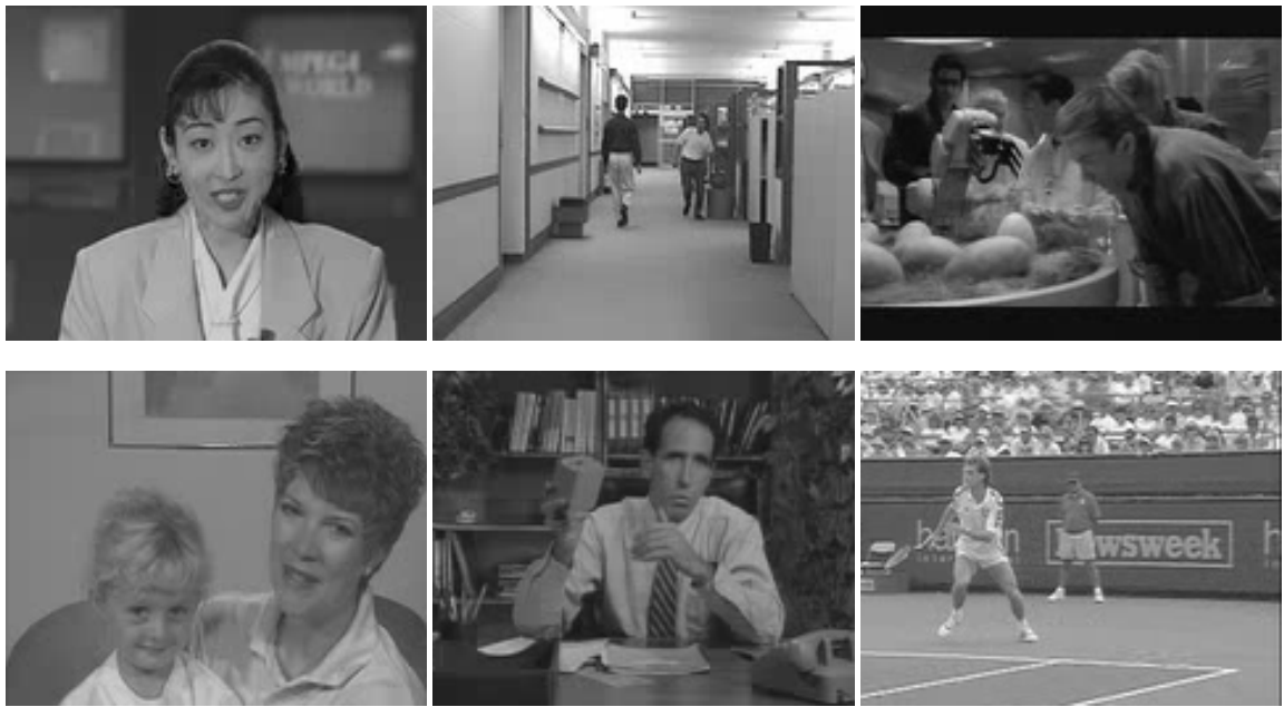
Figure 53: The tenth frame of the images, Akiyo, Hall, Jurassic, Mother and Daughter, Salesman and Stefan at the presentation level 18_4 at the packet loss of 5%.
