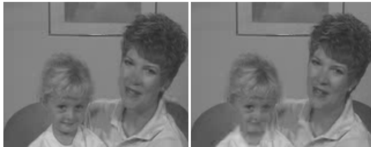
Figure 4: The tenth frame of the Mother and Daughter image at the presentation level 18_4 for the 20% and 35% packet loss, left and right respectively.
