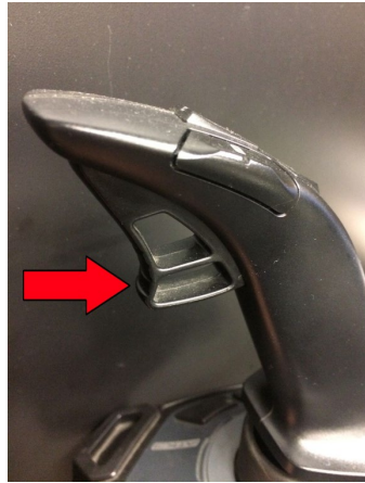
Fig. 4. Trigger to set current forward speed.
