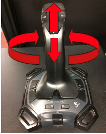
Fig. 3. Flight Mode Stick inputs.
